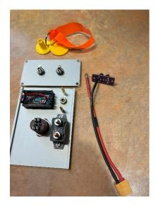
7. Cut a 4" piece of 16 gauge wire (negative) and strip about ¼" from each end. Then solder one end of that wire and the negative wire from the battery level meter to the Safety Key circuit board. Both these wires will be soldered in from the underside of the circuit board. Use to fastening nuts to mount the circuit board. The metal of the banana socket cannot touch both connectors. If they do, file down the excess.
