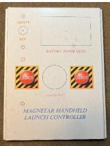
2. Drill all the holes, noted by a red + shape. For the rectangular hole, you will need to drill two large drill holes up to  $\frac{1}{2}$ " in diameter on each side of the + symbol, then use a mini hacksaw and a file to get the hole shape.
