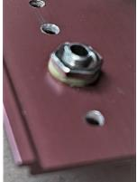
4. Install the launch push button switch and the battery level indicator on the top panel, and then mount two 4mm banana sockets on the front panel. The NC side of the switch needs to face Left.
