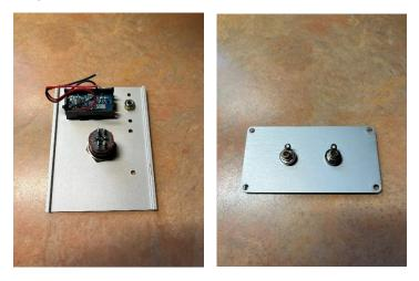
5. Assemble the Safety Key circuit board by mounting the battery clips and soldering them in place. Then cut one of the battery extension cables, leaving six inches of wire behind the male connector (mates with the battery connector). Strip ¼" from both red and black wires and dip the copper strands in solder flux. Solder the black wire into the Safety Key circuit board from underneath as shown.
