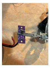
6. Screw in the 20 amp self-resetting fuse, placing a small #4 washer between the plastic housing and the fastening nut. Then screw in two 15mm standoffs for the Safety Key circuit board.
